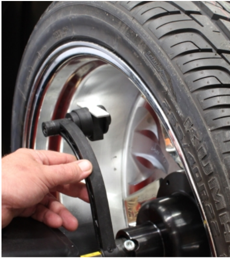
Precision Stick-On Weight Placement with ALU Data Arm
