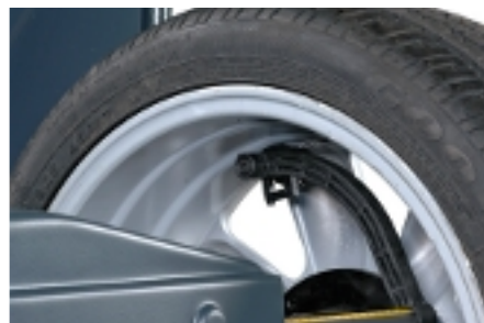
Precision Stick On Weight Placement With ALU Data Arm
