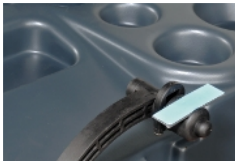
Precision Stick On Weight Placement With ALU Data Arm
